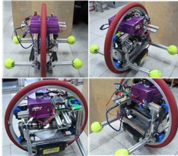
Fig. 7 Balancing demonstration of using roll and yaw angle control
