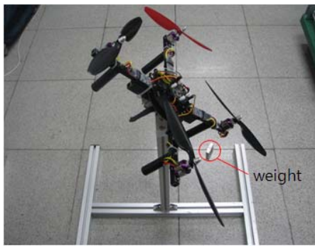
Fig. 6 Quad-rotor system test-bed
